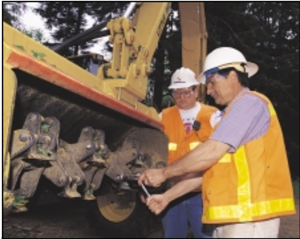
While ODOT group coordinator Nells Osterholme looks on, one of the nine men of Humbug Station, Tony Wiseman, tightens the knives of the Cat IT14G flail cutter head.
